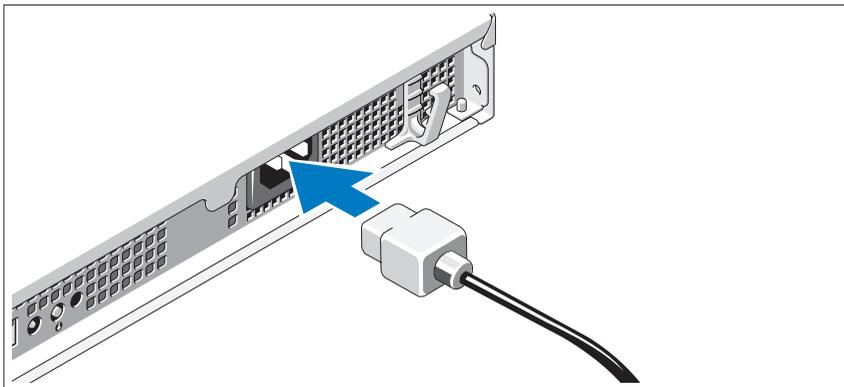
Connect the system's power cable to the system and, if a monitor is used, connect the monitor's power cable to the monitor.
