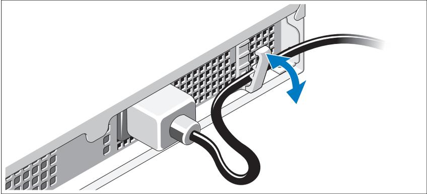
Bend the system power cable as shown in the illustration and secure the cable in the retention clip.
